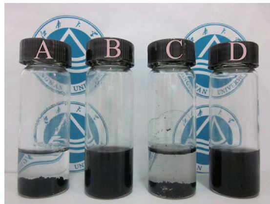
Figure 4. Aqueous dispersions of 0.5 wt% SWCNT-OH (A) without any dispersants (B) with P(St/VM-co-MA), and of 0.5 wt% MCWNT-OH (C) without any dispersants (D) with P(St/VM-co-MA). CNT:P(St/VM-co-MA) = 1:1 (weight ratio). The images were taken after 3 months storage.
